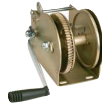
Ratchet winch (page 4) Reversible ratchet 1, 2 or 3 speeds. Removable handle.
